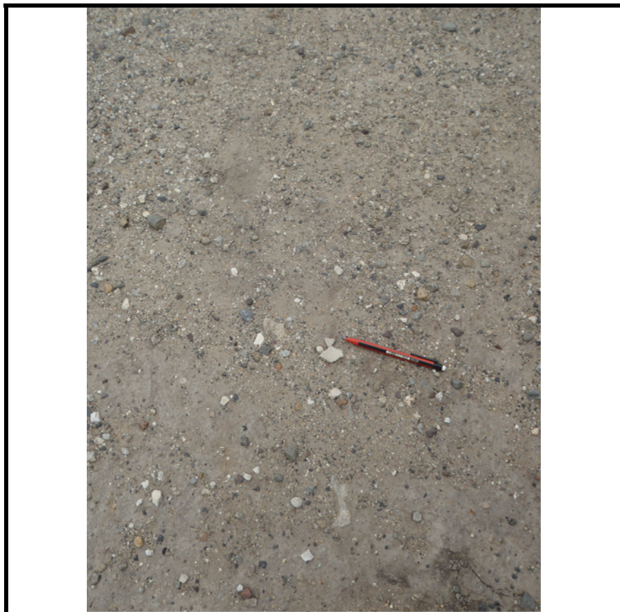
Photo 4: Example of ACM fragments in gravel road in the east of the speedway property
